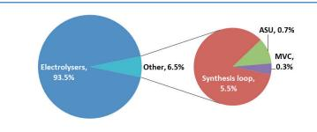
Figure 10. Indicative breakdowns of a large-scale all-electric ammonia plant's power needs
