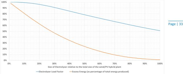
Figure 11. Electrolyser relative size, curtailment and load factors: The case of South Africa
