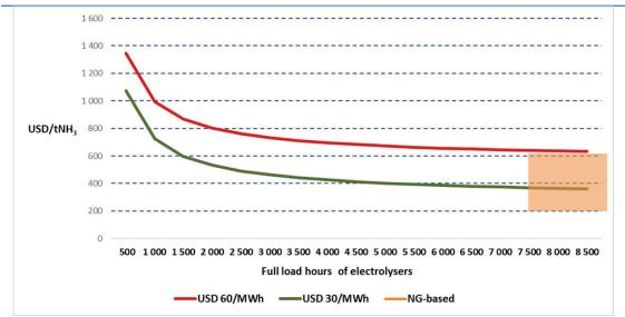
Figure 12. Cost of ammonia at various electricity prices and electrolyser load factors
